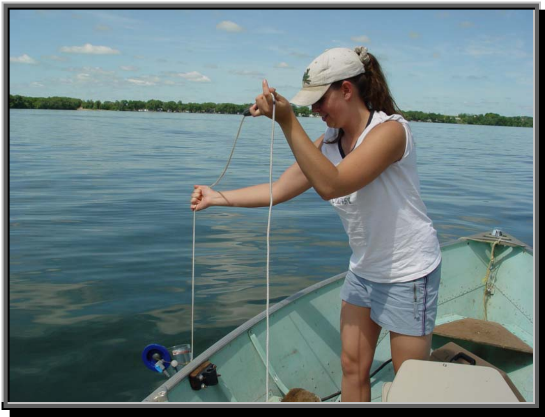
Figure 15. SDSU grad student using a VanDorn Collection Bottle while sampling Enemy Swim Lake during 2004.
